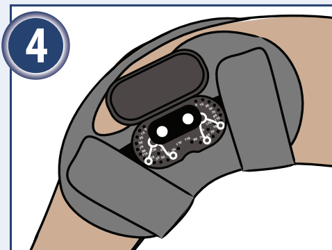
To adjust flexion and extension control, remove the pins to the desired settings of your prescribing physician.
